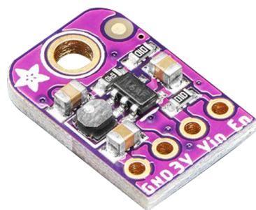
The AP3429A buck converter breakout features a 1.5MHz switching frequency, 100% duty cycle operation, thermal shutdown, and 35 $\mu$ A Quiescent current. This buck converter has a TLV62569 3.3V chip, and the PCB comes in Blinka-purple with a 2oz copper layer on top and bottom for better current carrying capabilities.
