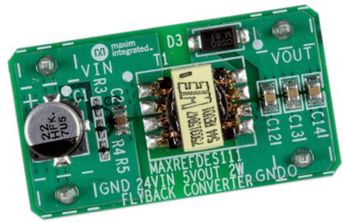
The MAXREFDES111 reference designs feature the MAX17498B, a peak-current-mode converter with an internal n-channel MOSFET switch. These reference designs can be used in the applications such as industrial control and automation, process control, telecom, and datacom power supplies.
