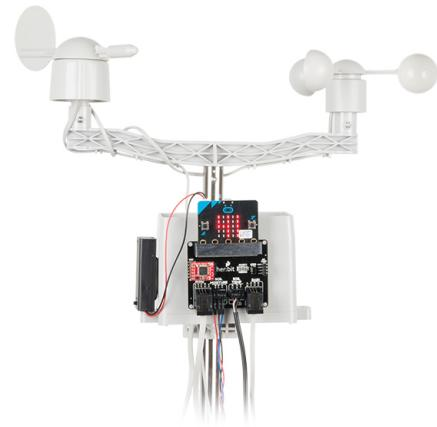
Inside each micro:climate kit the users will find all the components required to build micro:bit into a go-to weather sensor. The only parts not included are two AAA batteries, microSD card, and the micro:bit itself. Simply add the micro:bit to the provided weather:bit, assemble the kit, and you will be ready to start sensing. The SparkFun micro:climate kit is a great way to get your feet wet in high-grade sensors.
