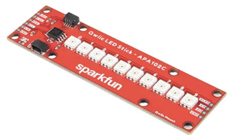
This board is one of SparkFun's many Qwiic compatible boards. Simply plug and go, no soldering, no figuring out which is SDA or SCL, and no voltage regulation or translation required.
