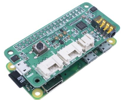
The ReSpeaker 2-Mics Pi HAT is designed based on the low-power stereo codec with 1W stereo class D speaker drivers developed for digital audio applications and cirrus logic WM8960. Other hardware includes 3 APA102 RGB LEDs, 1 User Button, 2 onboard grove interfaces for Expansion, and 2 microphones on both sides of the board for collecting sounds. The audio output is available through the 3.5mm audio jack or JST 2.0 speaker out.
