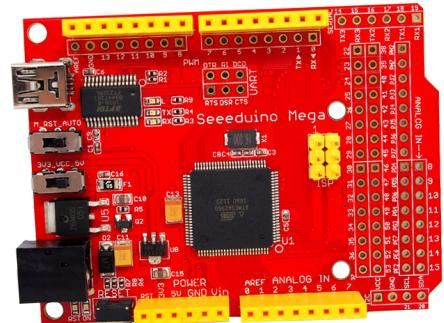
The Seeeduino Mega inherits deliberate details from Seeeduino, like selectable operating voltage (3.3V/5V), right angle reset button, and so on. This Seeeduino Mega is easy to program, no additional hardware is required to load firmware, just plug to a USB port and you're good to go. The device can be powered through a battery or through an AC to DC adaptor.
