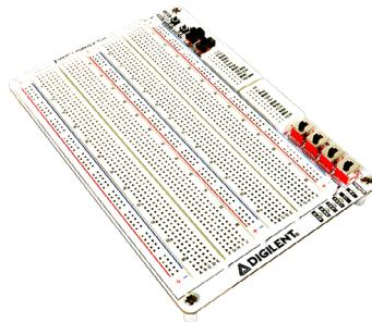
Each power supply can be switched on and off through slide switches to make powering on and off circuits as convenient as possible. The status of the power supply is indicated by the power indicator LEDs.
