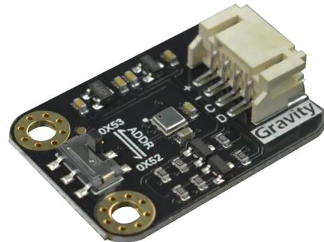
With intelligent on-chip algorithms, the ENS160 sensor can directly output rich and easy-to-understand environmental data.
