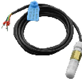
The SHT31 sensor offers high reliability and long-term stability with low power consumption, fast response, and strong anti-interference ability. The sensor supports I<sup>2</sup>C communication and is compatible with 3.3V/5V controllers like Arduino, micro:bit, and ESP32. The SHT31 is the standard version of the SHT3x series. It provides humidity accuracy of  $\pm 2\%$  RH @ 0% RH ~ 100% RH (at 25°C), and temperature accuracy of  $\pm 0.2^\circ\text{C}$  @ 0°C ~ 90°C (typical).
