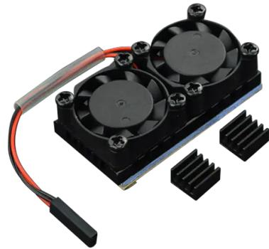
*Note: Clean the surface of the Raspberry Pi CPU, then tear off the adhesive film and stick the heat sink to the surface of the CPU, then you are good to go.*
