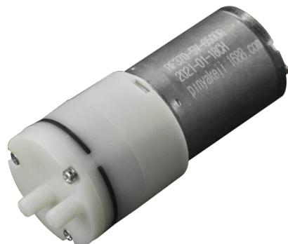
When powered on, the pump sucks air from the side port and outputs it from the middle port. The direction of the airflow can be changed by reversing the polarity of the motor. Two pumps are required to inflate and deflate at the same time. The pump flow rate is 2.2 Liters Per Minute (LPM), and its maximum suction is -58kpa. This air pump can be used in household appliances, medical equipment, vacuum packaging machines, and so on.
