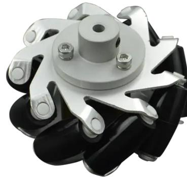
The Mecanum wheels feature a diameter of 65mm and are composed of 9 small rollers. These wheels are made of plastic and coated with quality and high-friction silicone rubber, which are rugged and impact-resistant. These Mecanum wheels feature better quality, texture and are equipped with a metal exterior structure that has its own coupling matching with various motor shafts. This makes it easy to install and ideal for smart robot cars.
