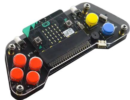
This gamepad features a programmable vibration motor, buzzer, and LED. The DFR0536 expansion board can be operated as a multimedia vibration controller or a multimedia interactive game console using graphical programming. The programming platform on the DFR0536 supports MakeCode graphical programming and python.
