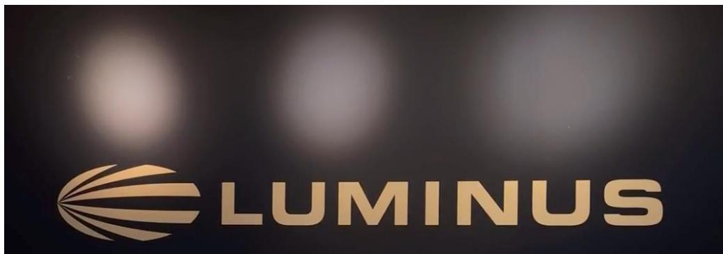
*The image above shows a beam comparison. On the left, a 4.5 mm Pico COB LES. In the center, a 6 mm LES. On the right, a 9 mm LES. Each COB is mounted into a PAR 20 lamp with identical optical systems, identical power, and they are producing the same lumens. Only the LES is different. We can clearly see that the 4.5 mm LES lamp produces more punch and a narrower beam.*
