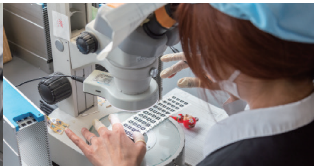
Processing accuracy is checked on each sensor using an electron microscope
