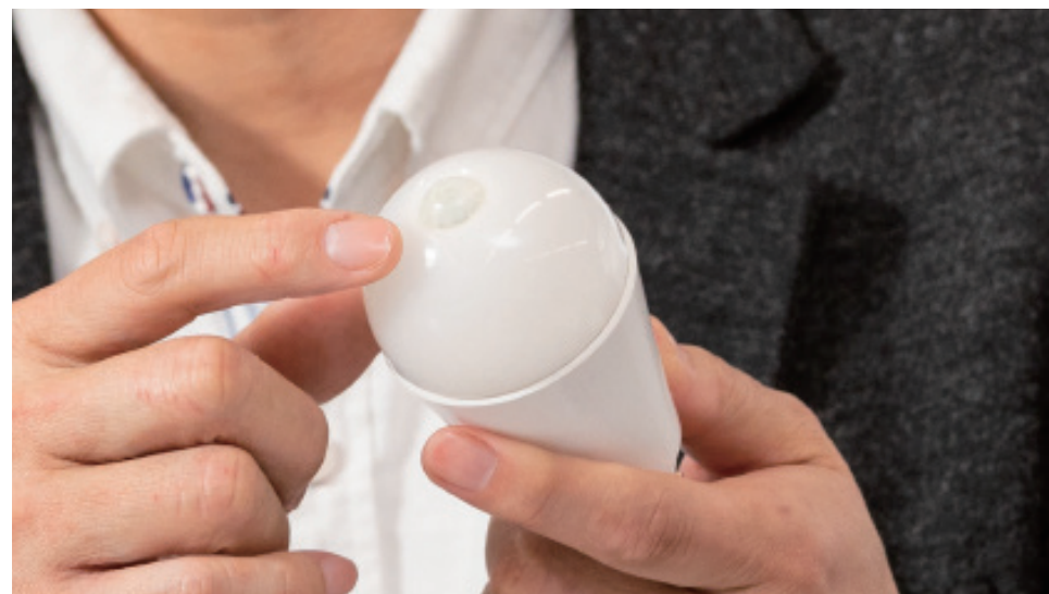
The lens is the protrusion in the center (motion sensor compatible lighting fixture)
