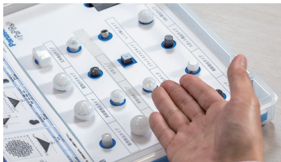
There are a total of 15 PaPIRs with different lenses
