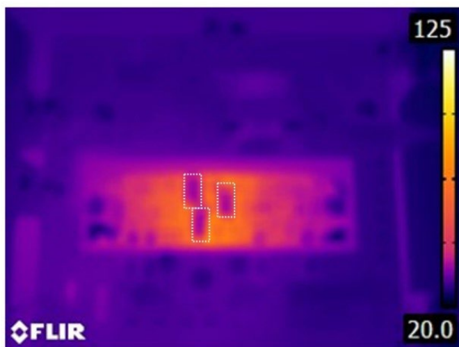
Figure 9: IR image of 100W MMIC without Q bridge (top), IR image of 100W MMIC with Q Bridge (bottom)
