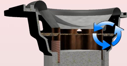
Air is forced into the magnetic loop on both sides of the voice coil for **10W** of continuous power and **20W** of peak power
