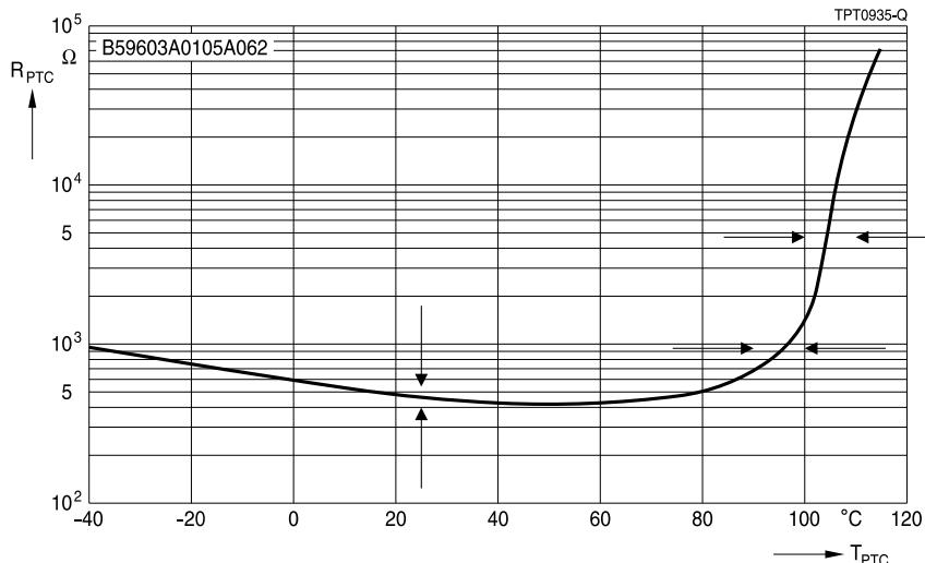
**Sensors****Limit temperature sensors, EIA case sizes 0402, 0603, 0805****Standard series****SMD****Characteristics (typical) for B59701A\*, EIA case size 0805**
