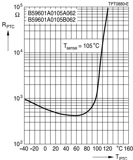
**Sensors****Limit temperature sensors, EIA case sizes 0402, 0603, 0805****Standard series****SMD****Characteristics (typical) for B59601A\*, EIA case size 0603**
