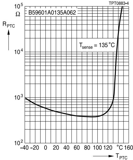
**Sensors****Limit temperature sensors, EIA case sizes 0402, 0603, 0805****Standard series****SMD****Characteristics (typical) for B59602A\* and B59603A\*, EIA case size 0603**
