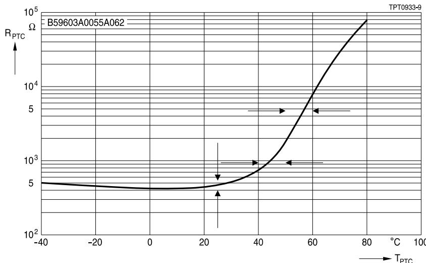
**Sensors****Limit temperature sensors, EIA case sizes 0402, 0603, 0805****Standard series****SMD****Characteristics (typical) for B59603A\*, EIA case size 0603**
