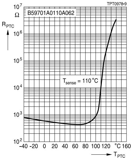
**Sensors****Limit temperature sensors, EIA case sizes 0402, 0603, 0805****Standard series****SMD****Characteristics (typical) for B59701A\*, EIA case size 0805**
