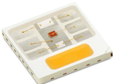
The LUXEON MultiColor Module 2.5W is a 4-in-1 package that makes color tuning easier. Each channel is individually addressable, enabling a large color gamut while simplifying the ability of getting just the right color point.
