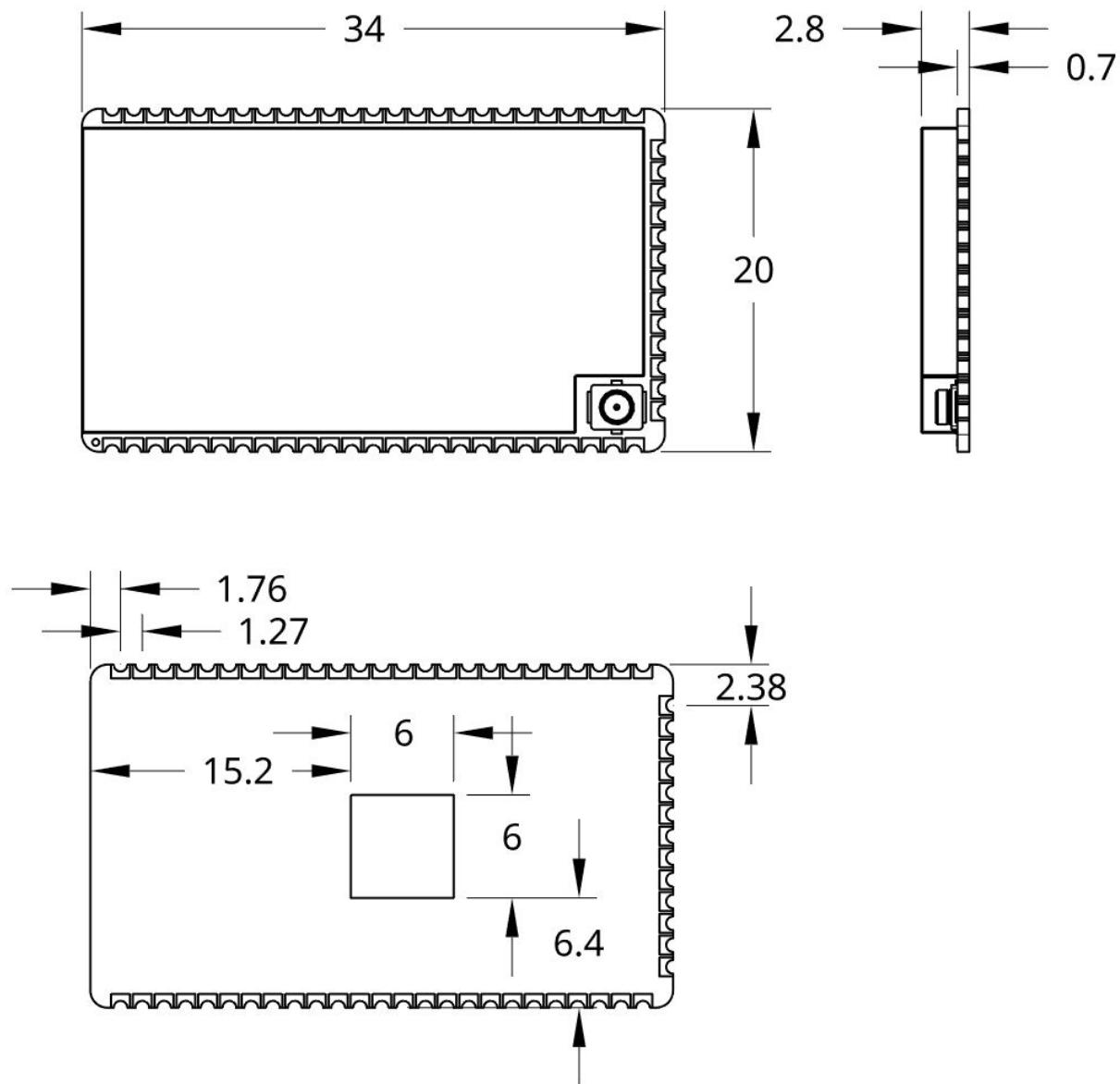
\* All measurements in millimeters
