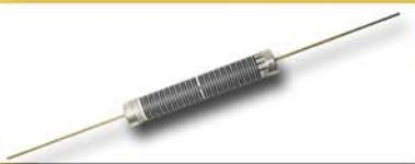
**Super MOX** High voltage SuperMOX resistors have been developed to meet the precision temperature stability requirements of high accuracy and high voltage systems. Super MOX combines a proprietary non-inductive system resistance and design to achieve a low temperature coefficient, low voltage coefficients, high stability and increase high operating voltages.
