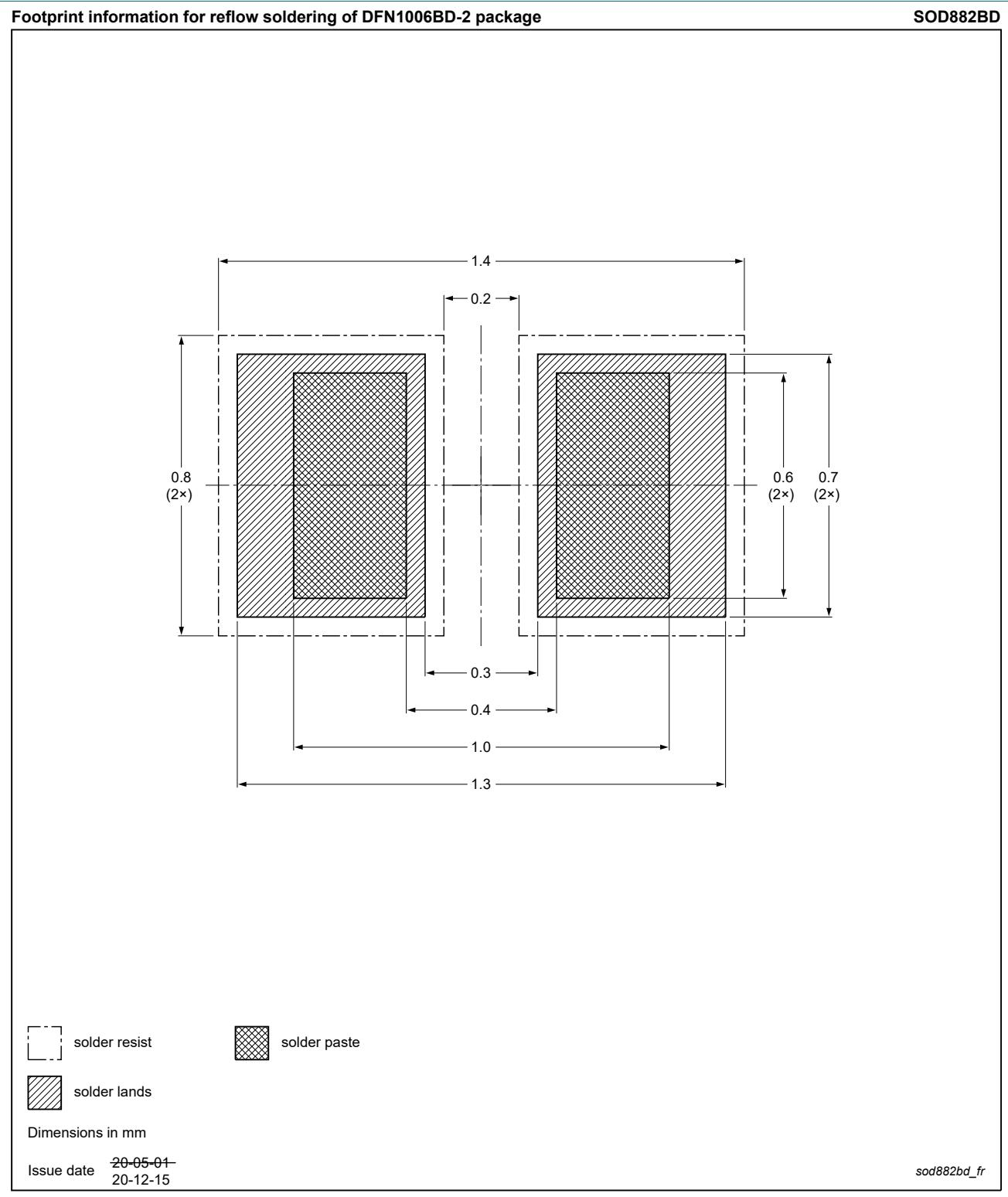
Fig. 2. Reflow soldering footprint for DFN1006BD-2 (SOD882BD)
