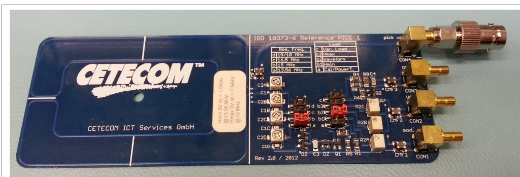
Figure 4. ISO/IEC 10373-6 Reference PICC Class 1
