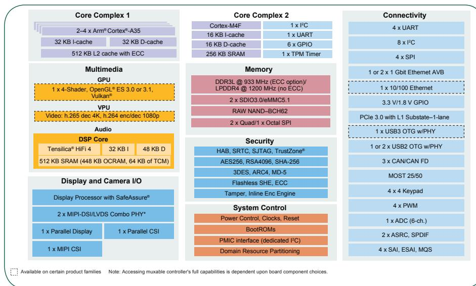
\* Each single PHY can either be a 1 x 4 lane MIPI-DSI or a 1 x 1 channel LVDS interface for a total of 2 display interfaces. In combination, the two PHYs can be configured to be a single 2-channel LVDS interface.
