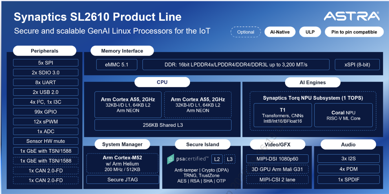
Figure 1. SL2610 Product Line of SoCs high-level block diagram
