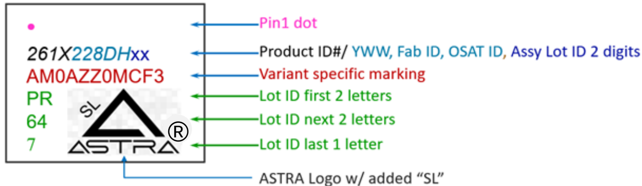
Figure 33. Package Marking and Pin 1 Location
