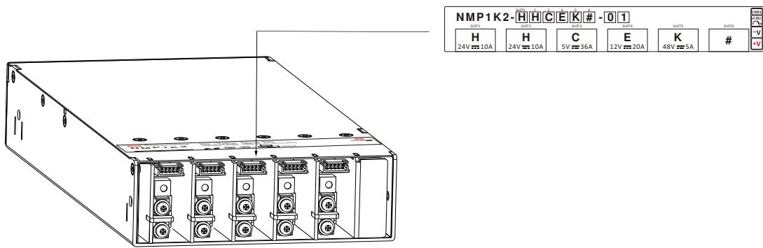
e. Apply AC power to the NMP unit, and measure the output voltages to ensure each module is functioning properly. Also, make sure the output voltage difference between slot 1 and slot 2 is less than 0.2V.
