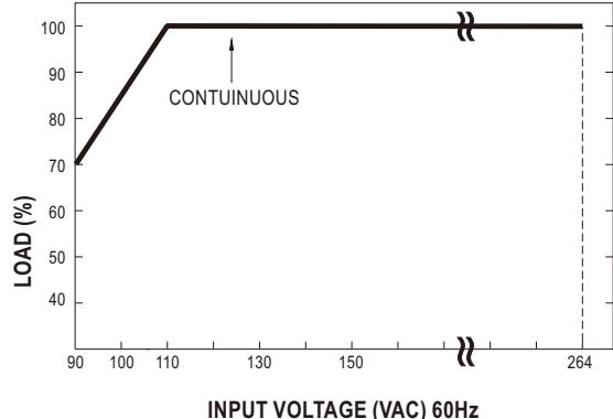
Figure 7-2 NMP1K2/NMP650 de-rating curves
