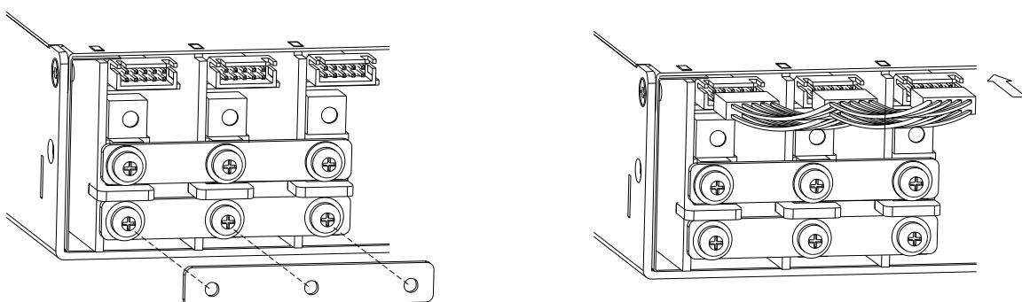
Recommended torque setting for output terminal screws is 6kgf-cm
