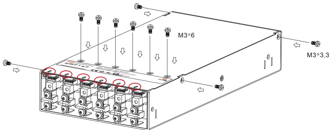
Note: Make sure all modules are slotted into the notches circled in red
