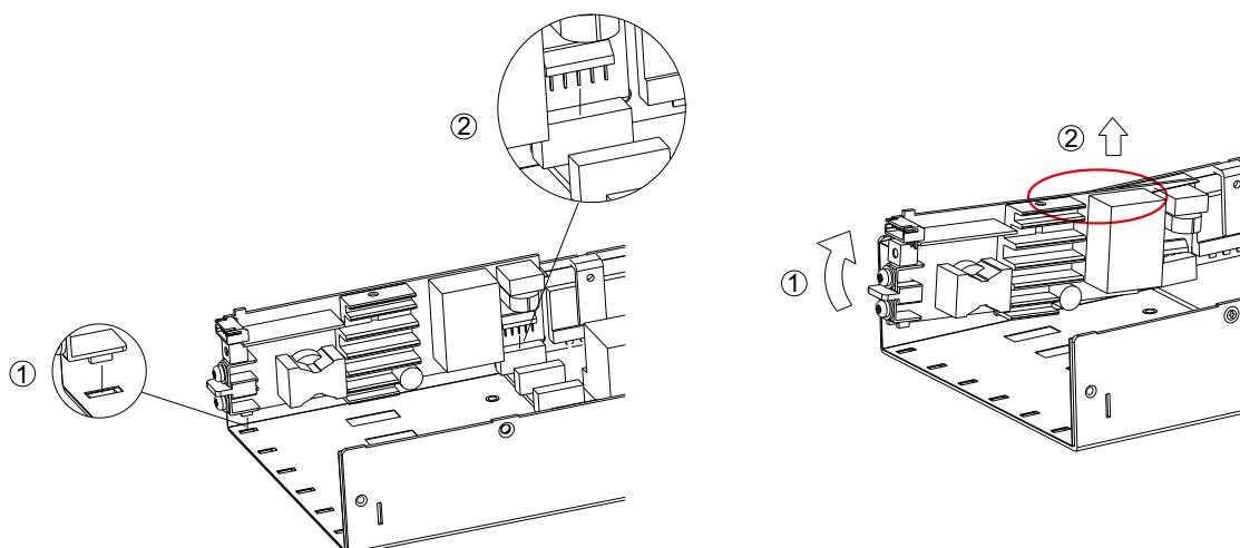
Install: ① Insert each module in a straight and leveled manner.
