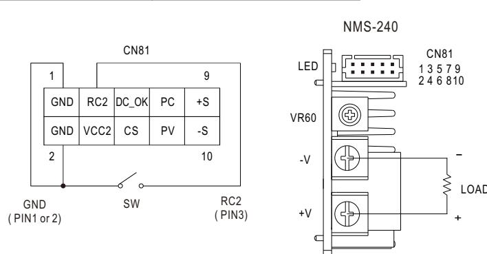
※ The CN32 connection accessory (included in packaging) must be connected when using the local ON/OFF function.
