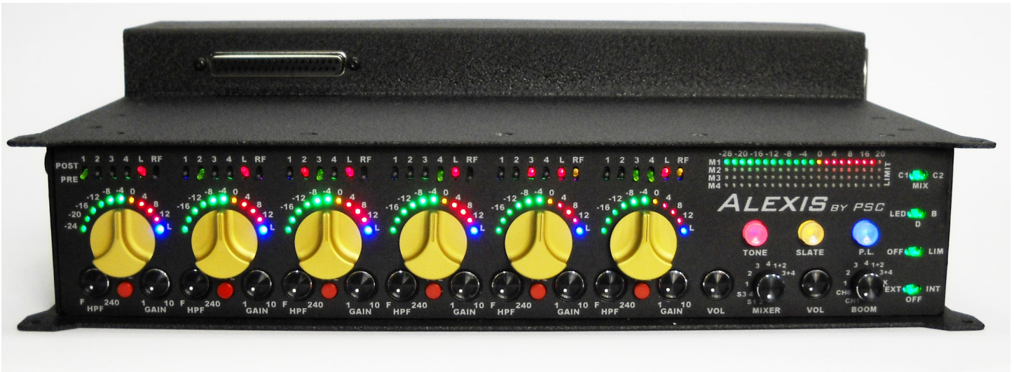
Figure 1: The Alexis Sound Mixer by the Professional Sound Corporation (PSC). It features NKK's B and G Series toggle switches.
