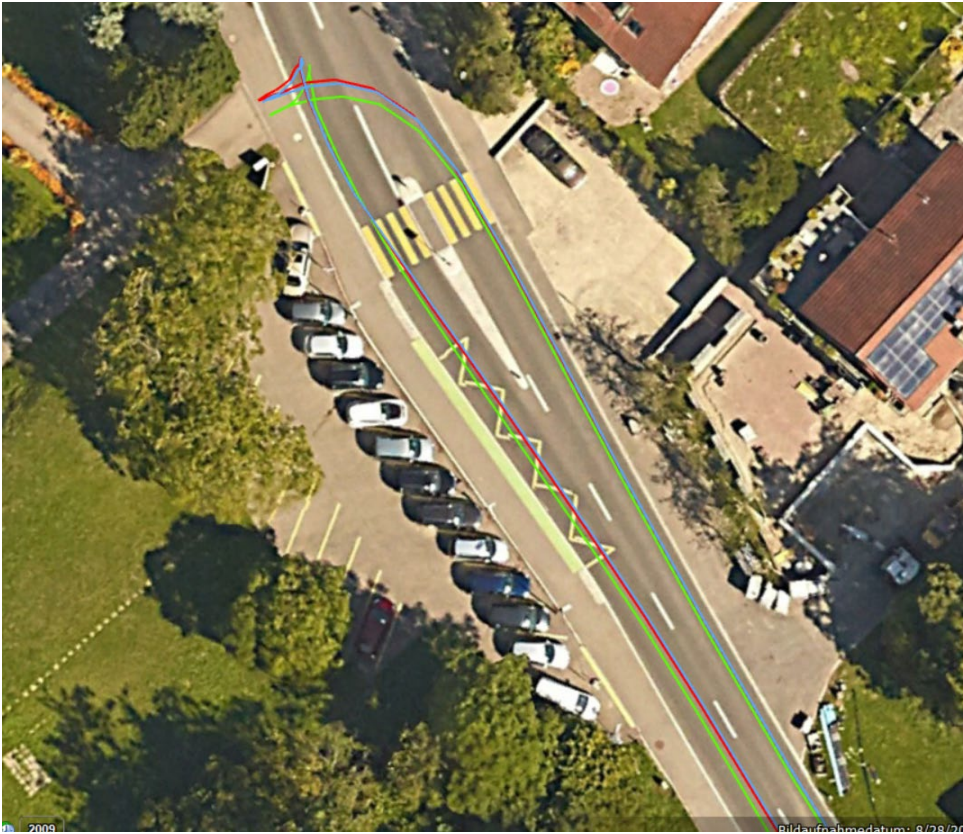
Figure 7: NEO-M8(Q/N), NEO-M8M, and reference position tracks in rural areas while changing heading of motion
