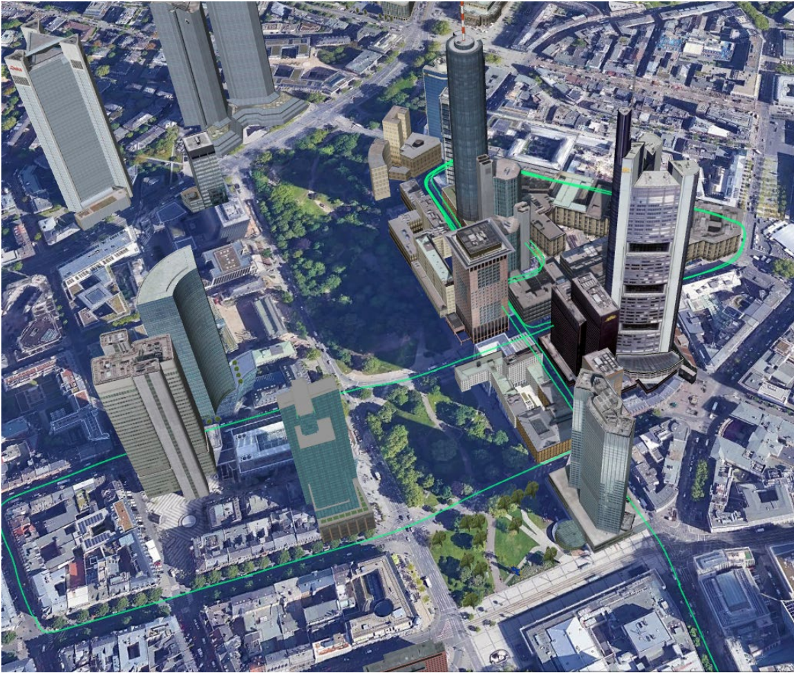
Figure 11: Scenario used for urban canyon to compare performance between NEO-M8(Q/N) and NEO-M8M
