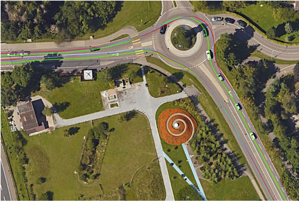
Figure 9: NEO-M8(Q/N), NEO-M8M, and reference position tracks in rural areas in a roundabout
