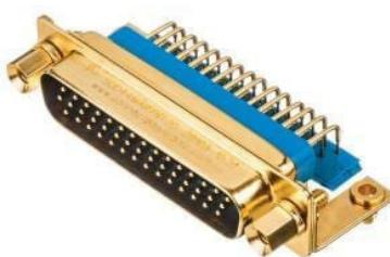
High performance D-Sub Connectors available in standard, high, and combination densities for applications requiring non-outgassing and low magnetism. All products conform to performance requirements of one or more of the following: MIL-DTL-24308, MIL-C-28748, SAE AS39029, GSFC S-311-P-4, GSFC S-311-P-10 and DSCC 85039.
