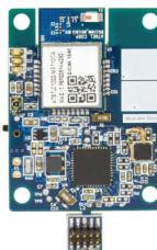
This board driven by SAML21 MCU is packed with sensors and BTLC1000 module on a tiny form factor PCB (40 x 30 mm) to demonstrate the ultra low power capabilities of SAML21 for wearable applications. It runs on coin cell battery and comes with a free android app to provide 3D plot, step count, motion and environment sensing information.
