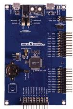
The SAML21 Xplained Pro Evaluation Kit is ideal for evaluating and prototyping with the ultra-low power SAML21 ARM Cortex-M0+ based microcontrollers.
