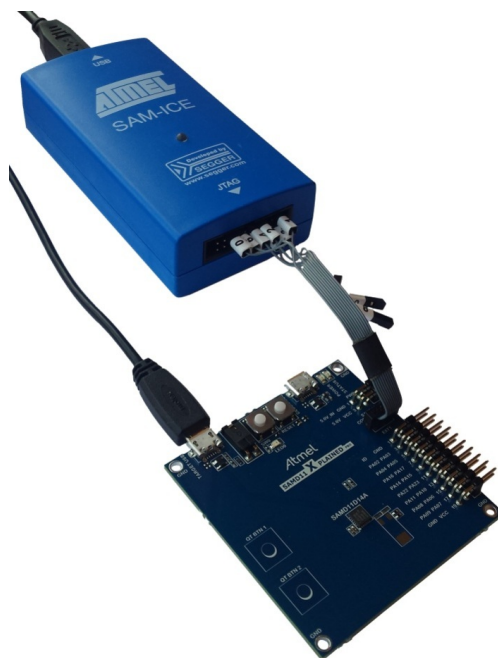
Figure 7-2. SAM-ICE using an Atmel-ICE Adapter
