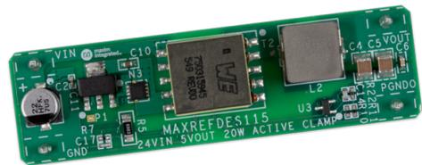
Each of the MAXREFDES115 isolated power supply reference designs has been tested for load and line regulation, as well as efficiency and transient performance. The MAXREFDES115 is an efficient active clamp topology with 24V input and a 5V output at 4A (20W) of power. The design features the MAX17599, a low-IQ wide-input-range active-clamp current-mode PWM controller. This entire circuit fits on a 20mm x 55mm board.
