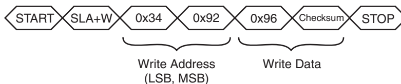
FIGURE 4: EXAMPLE OF A WRITE TO ADDRESS 0X1234 WITH A CHECKSUM
