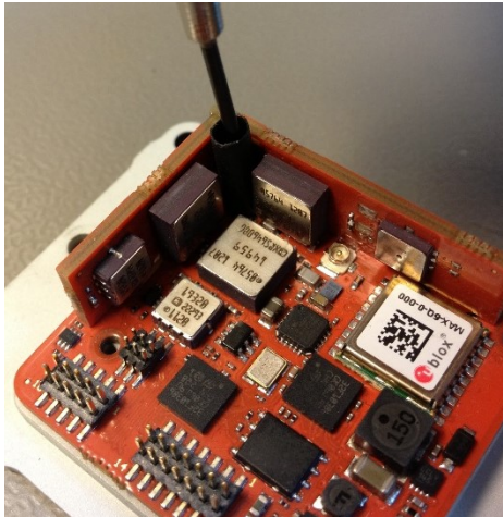
Figure 14: Using a heat shrink tube to position the mounting screws
