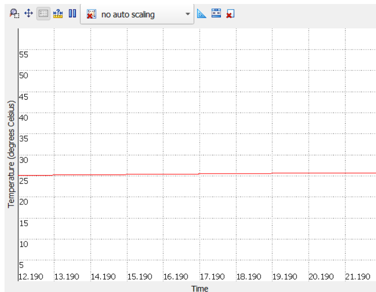
Figure 34: The Temperature view window, showing that the MTi is warming up directly after powering it.
