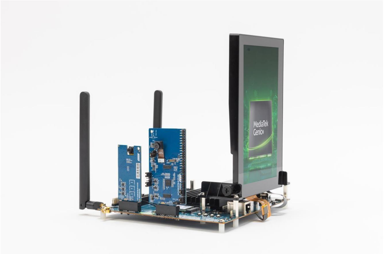
Figure 2-1. Genio 700 (MT8390) EVK Board System Setup
