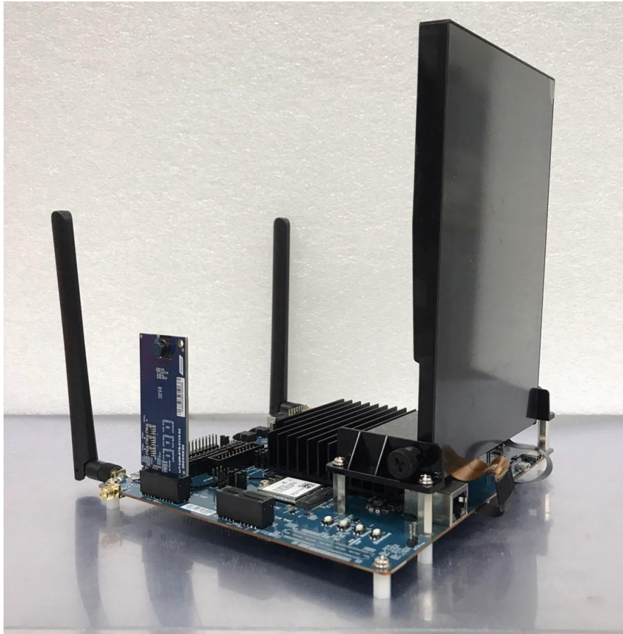
Figure 2-1. Genio 510 (MT8370) EVK Board System Setup
