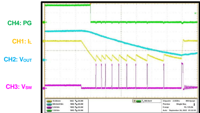
OVP/NOCP OVP level = 130% of VID, NOCP = -20A, OVP trigger delay = 1μs, hiccup mode
