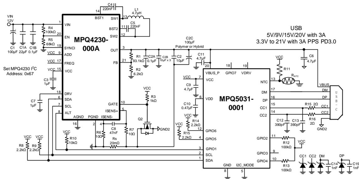
Figure 5:  $V_{IN} = 12V$ ,  $V_{OUT} = 3.3V$  to  $21V$  for USB PD and PPS Applications
