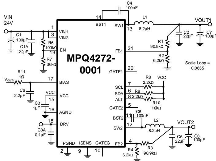
Figure 3:  $V_{IN} = 24V$ ,  $V_{OUT1}$ ,  $V_{OUT2} = 3.3V$  to  $21V$ ,  $3A$  Load
