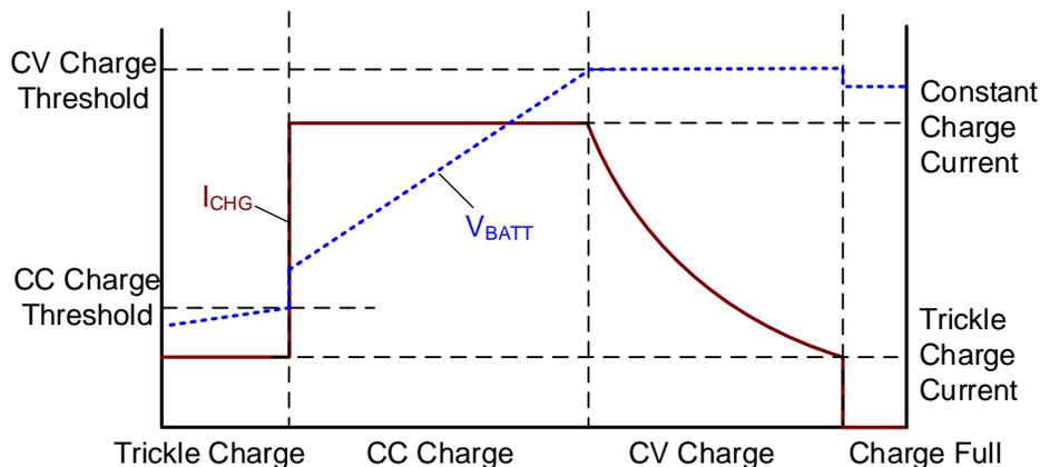
Figure 1: Lithium-Ion Charging Profile
