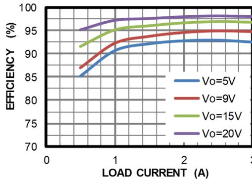
Figure 4: MPQ4272 Efficiency Curve
