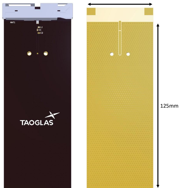
Top Side (MPA.66.A placement on 50x50mm PCB)
