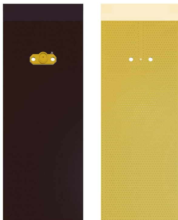
Bottom Side (MPA.66.A placement on 50x50mm PCB)
