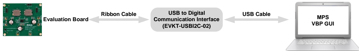
Figure 1: EVKT-MP4255 Evaluation Kit Set-Up
