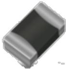
0603 to 1206 case size thermistors are widely used for temperature compensation as well as for temperature control of printed circuits in wide range of applications. Available with Ni barrier/100% Sn termination for lead free soldering or with PdAg termination for hybrid assembly.
