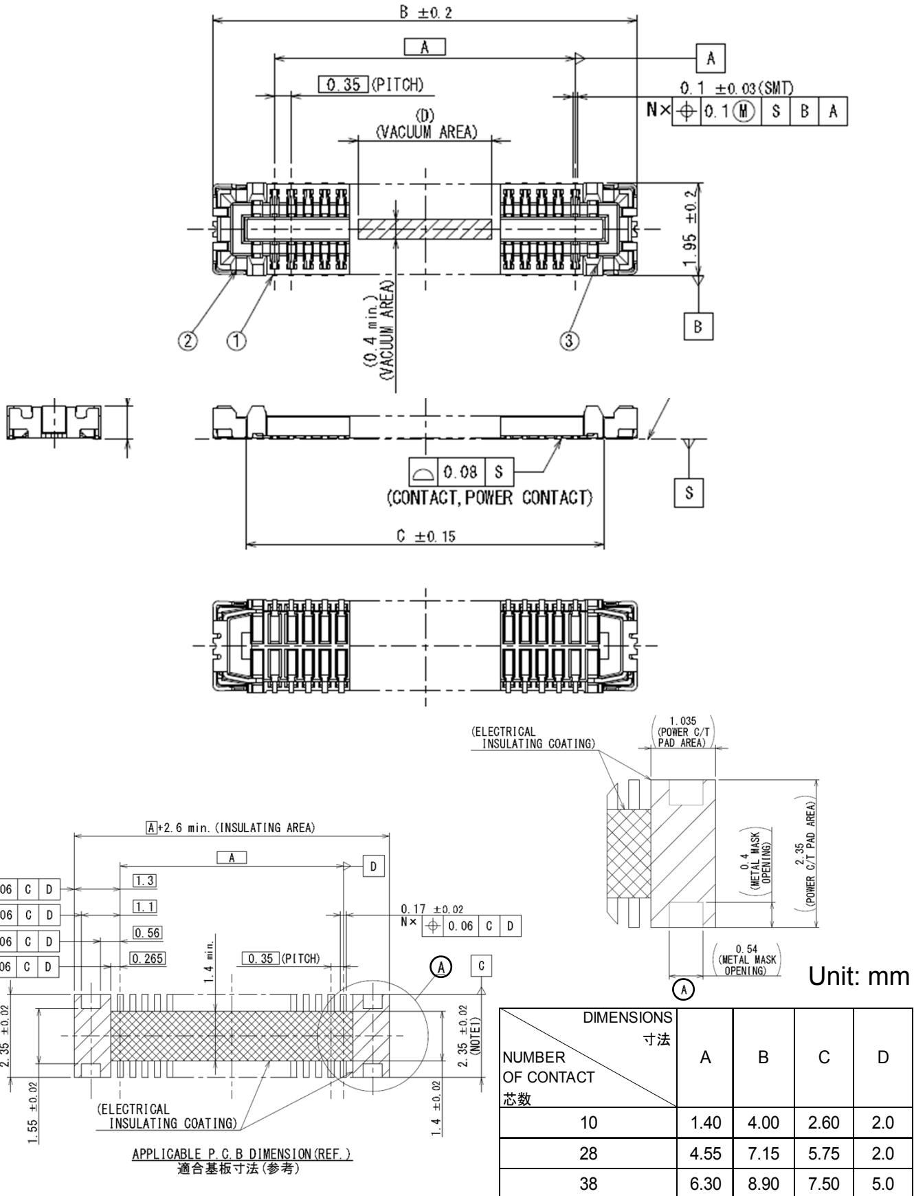
Note 1) Dimension  $2.95 \pm 0.05$  is recommended in case repair is needed.
