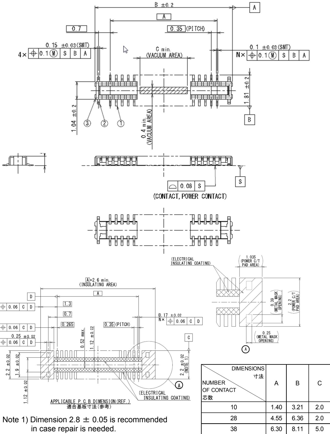
Note 1) Dimension  $2.8 \pm 0.05$  is recommended in case repair is needed.
