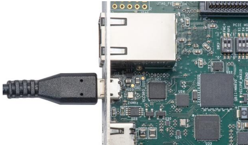
Figure 4-2 Connection setup for using dashboard system
