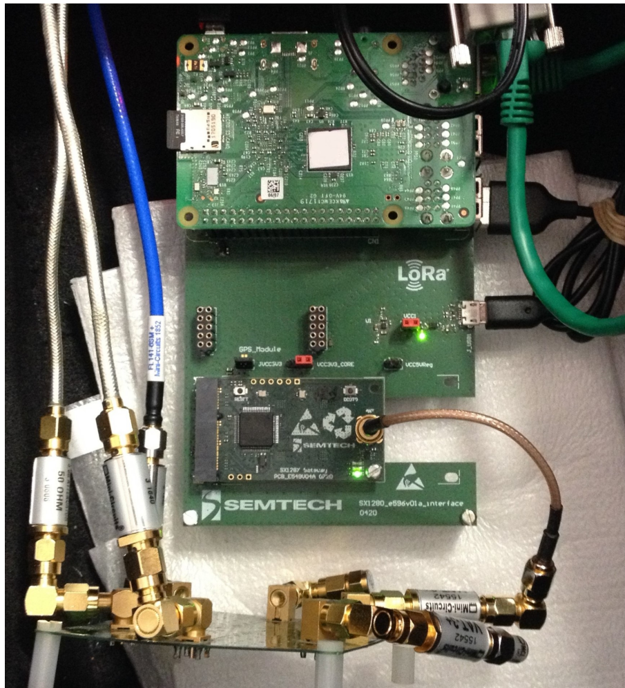
Figure 2.2: The power splitter, the RPI and the DUT are all enclosed in RF shield box to protect against real world
