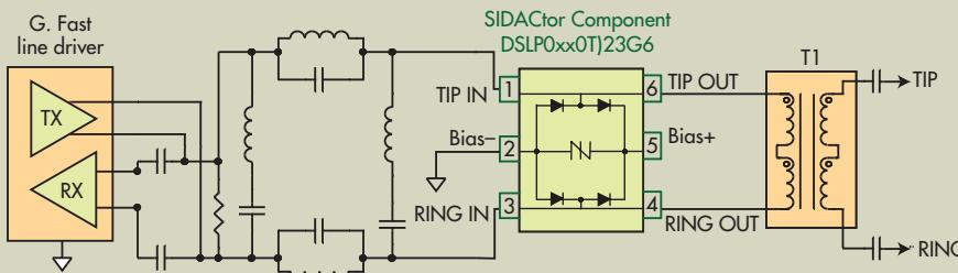
**2. The DSLO Biased Series provides a typical surge capacity of 35 Amps (8/20 µs) with only 1.3 pF of typical loading capacitance, and is packaged such that flow-through routing of the data tracks is possible.**
