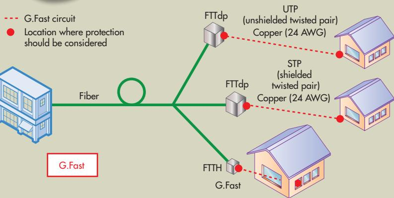
**1. In this implementation, service providers will use existing fiber optic cables to bring high-speed connections to transition points like FTTdp (Fiber To The Distribution Point) and FTTH (Fiber To The Home).**
