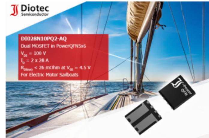
Two such parts in a H-bridge configuration are already enough to drive a brushed DC motor with adjustable speed and reversal of propulsion. Just three parts are enough to form a three-phase bridge capable for driving brushless DC motors (BLDC). The on-state resistance of typical 15 mOhm at 10 V Gate-Source voltage or maximum 26 mOhm at 4.5 V helps to save energy and therefore prolongs the runtime of the drive.
