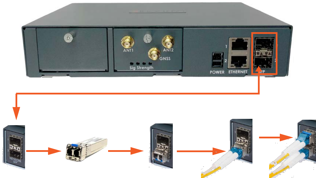
Figure 2-10 Dual SFP Connection. Inserting the SFP transceiver
