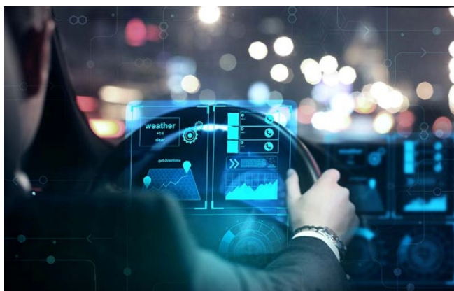
Heads-up displays project images on the windshield such as travel speed or directions from a GPS system.
