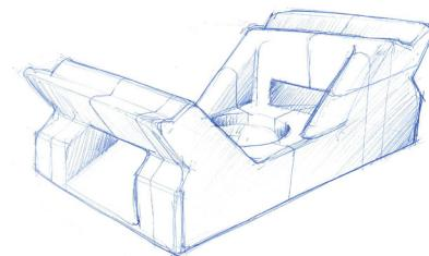
**Double saddles** firmly hold and separate wires (if wire separation is desired).
